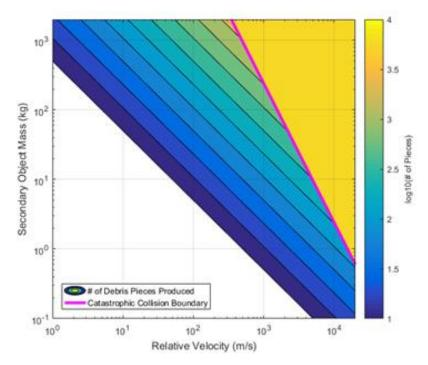
Figure O-1 Range of Debris Production Possibilities 16
