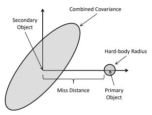
Figure N-4 Representation of the Conjunction Plane
