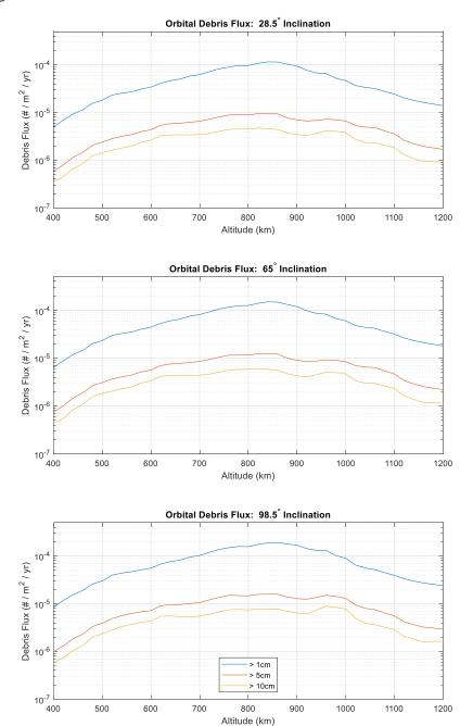
Figure G-1 Debris Flux as a Function of Orbit Inclination, Orbit Altitude, and Object Size
