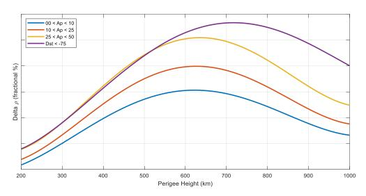
Figure N-7 Behavior of Relative Density Error by Perigee Height and Solar Activity
