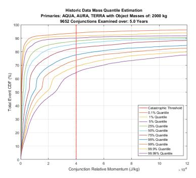
Figure O-3 Catastrophic/Non-Catastrophic Composition as a Function of Mass Quantile<sup>18</sup>
