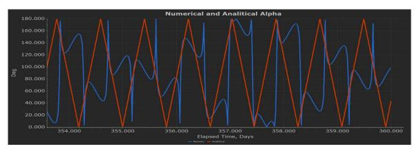
Figure H-2 Numerical vs. Analytic (Linear) α for Highly Eccentric Orbit
