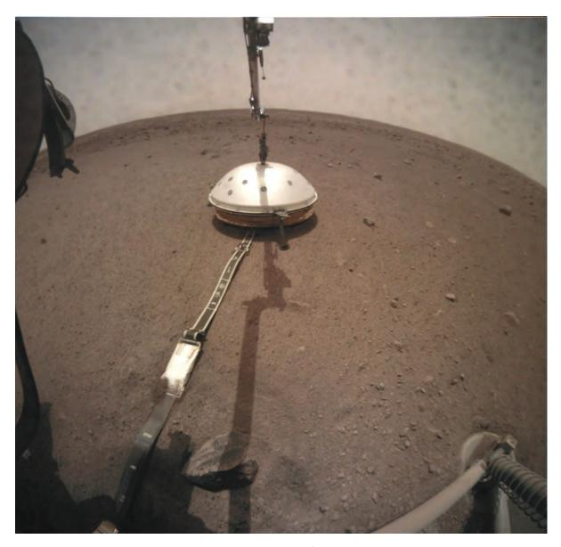
Deployment of the SEIS Protection Dome on Mars.
