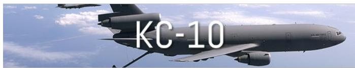
**What does it do?** The KC-10 is an aerial refueler that can carry up to 356,000 pounds of fuel, almost twice as much as the KC-135 tanker. Unlike most KC-135s, the KC-10 can refuel aircraft using a boom or drogue.
