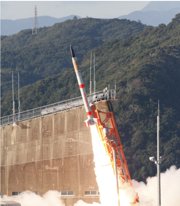
A test of the SS-520 rocket from the Uchinoura Space Center. The SS-520, a small sounding rocket, is the smallest launch vehicle to ever carry an object to orbit. Photo: JAXA
