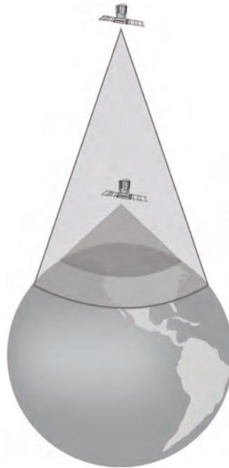
Table 5.1 lists the radius of the maximum observable ground area by satellites at several altitudes, and the radius of the effective ground area when the minimum elevation angle is  $10^\circ$ . Note that for satellites at low altitudes the effective area is roughly half of the maximum observable area, while for
