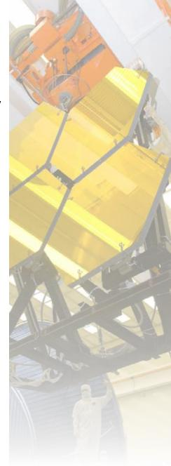
The James Webb Space Telescope mirrors have completed deepfreeze tests and are removed from the X-ray and Cryogenic test Facility at Marshall Space Flight Center. (NASA)
