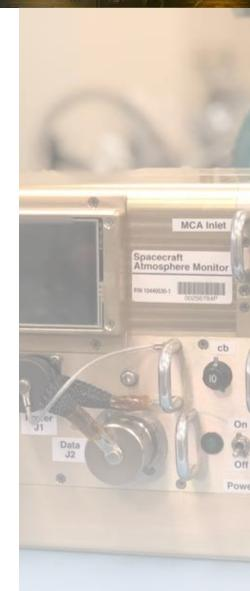
Spacecraft Atmosphere Monitor (SAM) is one of the smallest (mass and power) autonomous GCMS instruments ever built and will continuously monitor the major components found in air in real-time. (NASA)
