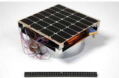
The Photovoltaic Radio-frequency Antenna Module (PRAM) with a 12-inch ruler for scale. The hardware is the first orbital experiment designed to convert sunlight for microwave power transmission for solar power satellites. (Source: US Naval Research Laboratory).
