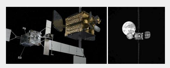
(Left) Artist's concept of Space Logistics mission extension vehicle (MEV-1) approaching IntelSat's IS-901 satellite to provide life extension - a first for the commercial space industry. (Right) Photo of IS-901 taken by MEV-1 just before docking on February 25 of this year. (Source: Northrop Grumman)
