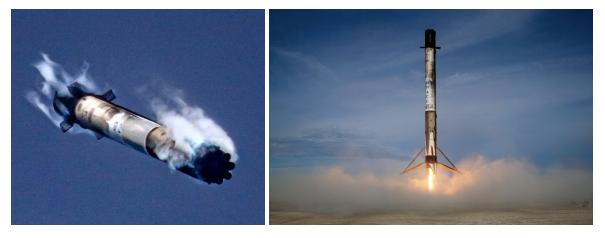
A Falcon 9 reusable first stage during hypersonic reentry and landing at Cape Canaveral, Florida on 25 July 2019. The same core was flown on 4 May 2019 - 82 days prior - and then refurbished. (Source: SpaceX)
